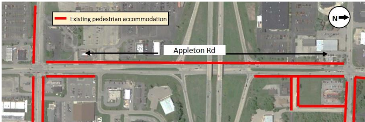
Figure 88. Existing (pre-construction) pedestrian accommodations at Appleton Road interchange. Source: UW-TOPS Lab
