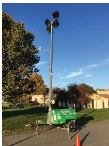
(a) Terex RL4000–Metal halide light tower
